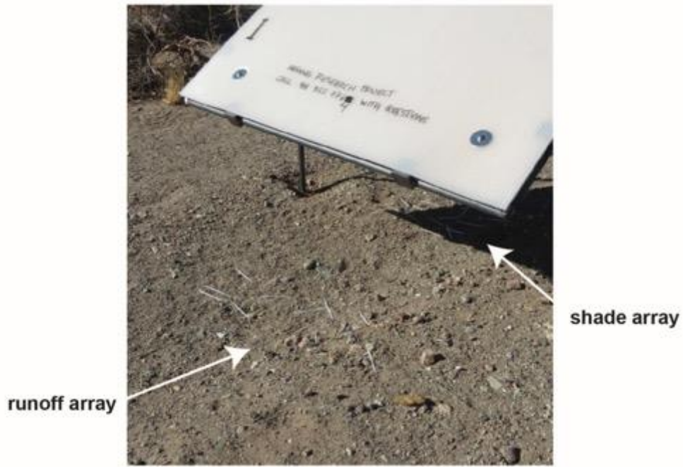
Figure B-11: Ant Disturbance of Toothpick Arrays
