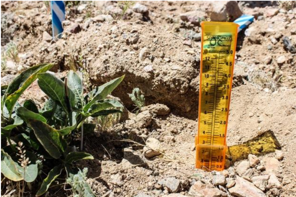
Figure 7: SoilDuck Temperature Sensor Installed under Mojave Milkweed
